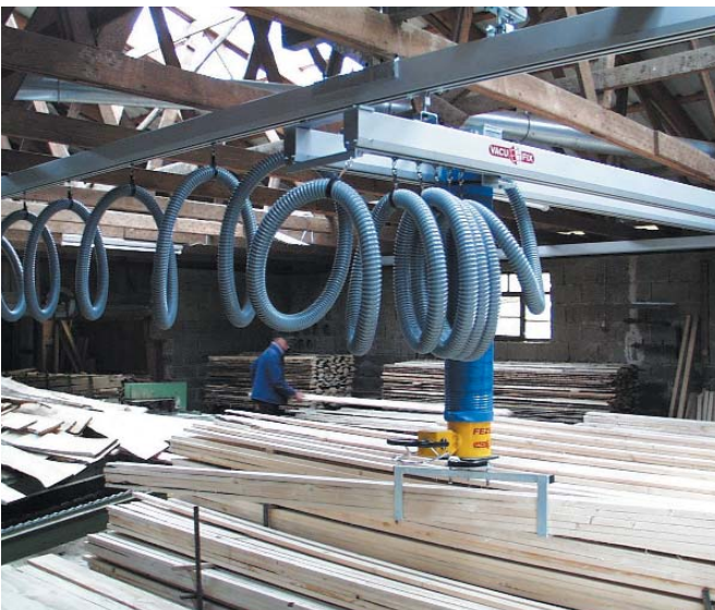
Suspension track system with ceiling suspension and double bridge. Work area: 10.000 x 8.000
