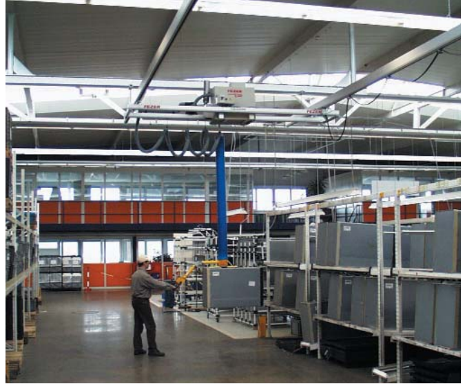
Suspension track system with ceiling suspension. Work area: 30.000 x 8.000
