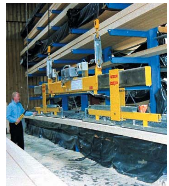
VWLB with safety feature to prevent device from tipping over
