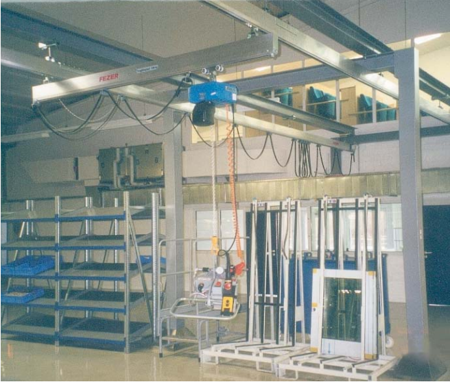
Suspension track system with portal construction. Work area: 10.000 x 4.000
