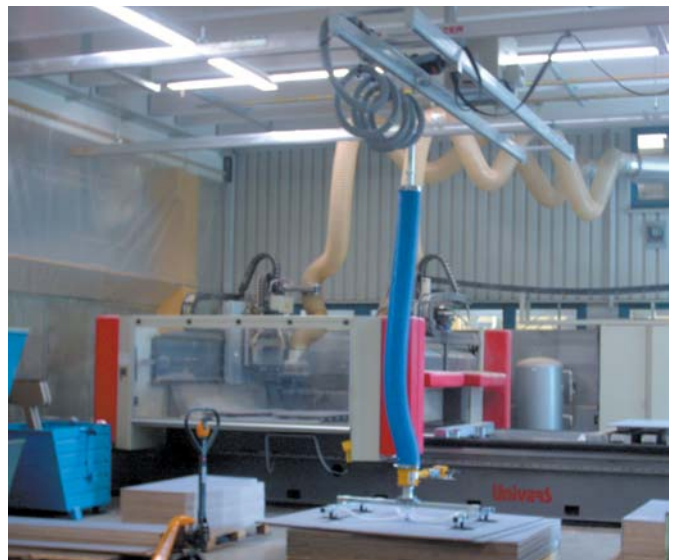
Suspension track system with ceiling suspension and double bridge. Work area: 8.000 x 5.000
