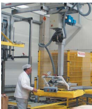
LiftFix with vacuum suction frame and frequency converter
