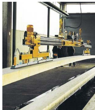
VWLB with motor-driven adjustable suction plates
