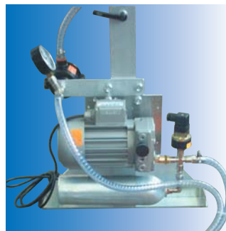
Vacuum generator with non-return valve, Eco-Module and safety tank
