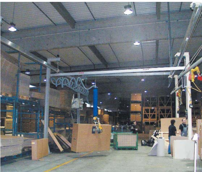
Suspension track system with portal construction. Work area: 18.000 x 7.000
