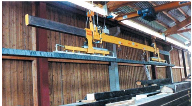
VWLB for gluelam beams wrapped in packing foil with a length of 20 metres and separate vacuum energy unit.
