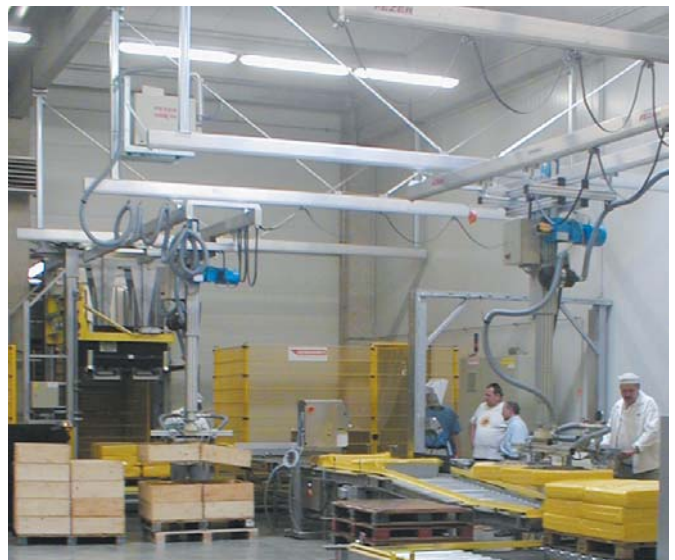
Suspension track system with ceiling suspension and rigid lifting unit "LiftFix". Work area: 2 x 6.000 x 5.000
