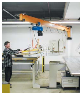
Wall Slewing Jib with chain hoist up to 250 kg
